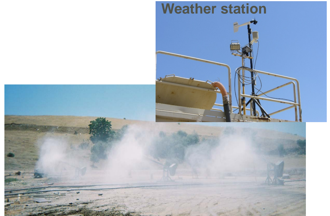
Three spray evaporators, in operation
